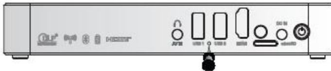
On the rear side of Qumi (below the two USB ports), there is a small pinhole. Insert a paperclip (or similar sized object) into the hole and press for 3 seconds to reboot Qumi.
