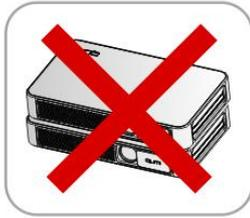
Make sure that the intake vents do not recycle hot air from the exhaust vent.
